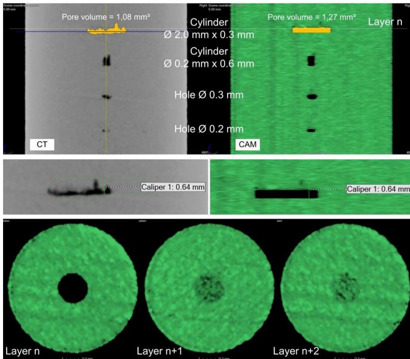
Figure 7. Cross-sectional views through the sample CL 31AL 1\_3 of BJ 2 with CT and CAM images from the side view (top), detail view of cylinder Ø 2.0 x 0.3 mm (middle) and view on three consecutive layers (bottom), whereby layer n is the last layer inside the cylinder Ø 2.0 x 0.3 mm and layer n+1 and layer n+2 are the first two layers with melt tracks above the cylinder.
