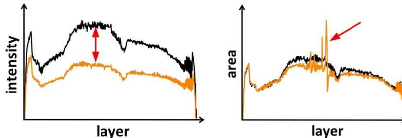
Figure 2. Melt pool intensity for two identical parts manufactured with different laser power (left chart) and modified powder dosing (layer thickness) in the middle layers (right chart).
