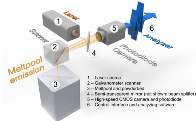
Figure 1. Principle and main components of QM Meltpool 3D system [11].
