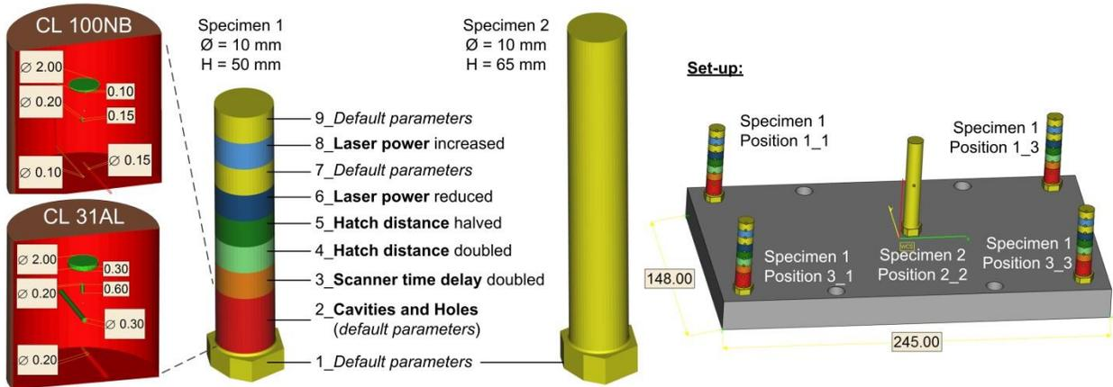
Figure 5. Design of specimen 1 and 2 (center) with detail view of section 2 of specimen 1 (left: magnified sectional view) and set-up of specimens on build platform (right) with sample ID.
