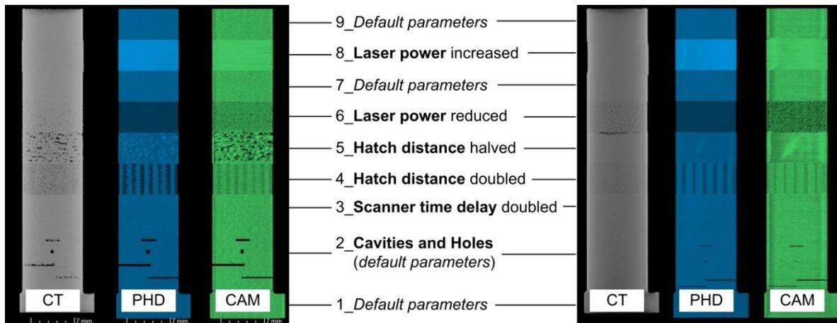
Figure 9. Cross-sectional views through the samples CL 31AL 1\_3 of BJ 2 (left) and CL 100NB 1\_3 of BJ 3 (right).
