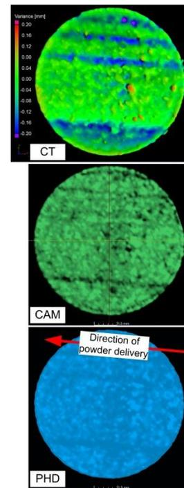
Figure 8. Geometric comparison of CT data to CAD (top) and corresponding top layer of CAM (middle) and PHD data (bottom), sample CL 31 AL 3\_1 BJ 3.
