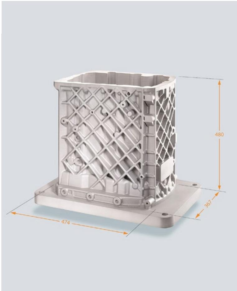
This gearbox is made of aluminium and manufactured on a Concept Laser X line 2000R machine. The material is CL 31AL (AlSi10Mg). Additive Manufacturing offered reductions in weight, cost and manufacturing time as well as giving the designer significant design freedom (Courtesy Concept Laser)
