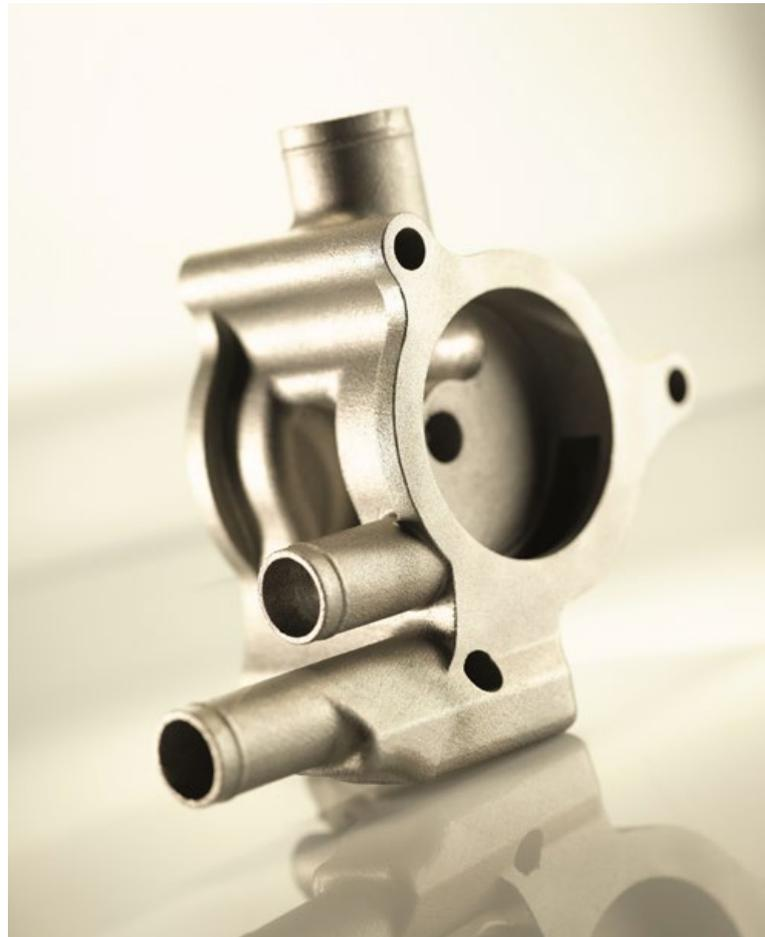
This oil pump housing is made of aluminium alloy and manufactured on a Concept Laser M2 cusing machine from CL 31AL (AlSi10Mg). As well as offering a reduction in manufacturing time, AM enabled an optimum design in terms of flow properties as there are no sharp-edged transitions as a result of drill holes (Courtesy Concept Laser)
