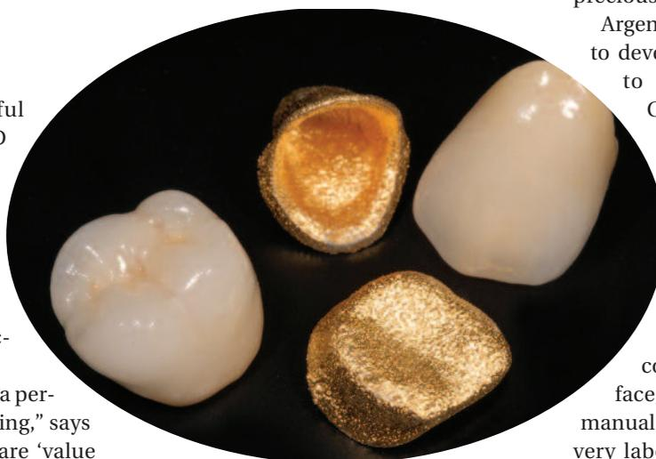
*The Argen SLMCaptek crown is printed on a Concept Laser Mlab machine, and then infiltrated with gold and veneered with porcelain.*
