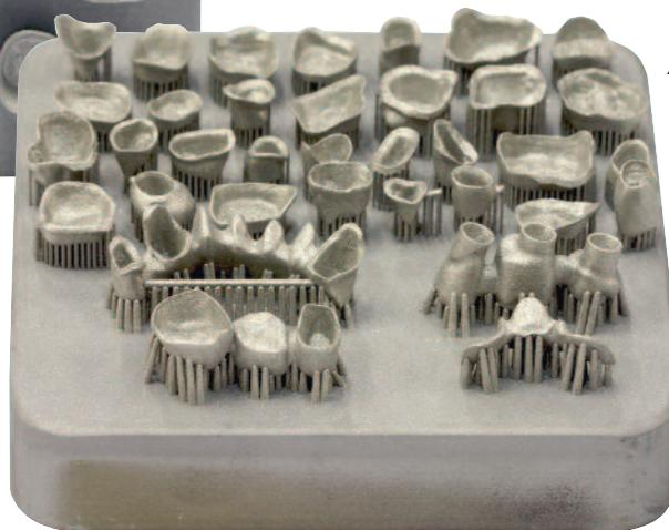
*Argen prints several crowns and bridges, shown here on a 90 by 90-mm build plate, per production cycle on its Concept Laser Mlab 3D metal-printing machines.*
