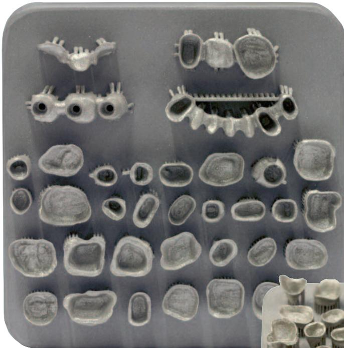
..thanks to digitization and quick-changeover 3D metal-printing machines. This industry-leading digital outsourcing center employs 16 metal-printing machines worldwide (12 at its manufacturing facility in Southern California) to keep up with growing demand for printed dental-restoration devices.
